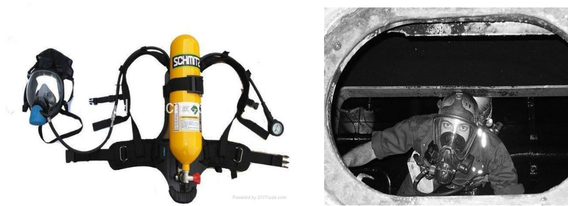
Fig. 5.2.4.C: Entering enclosed space with SCBA
