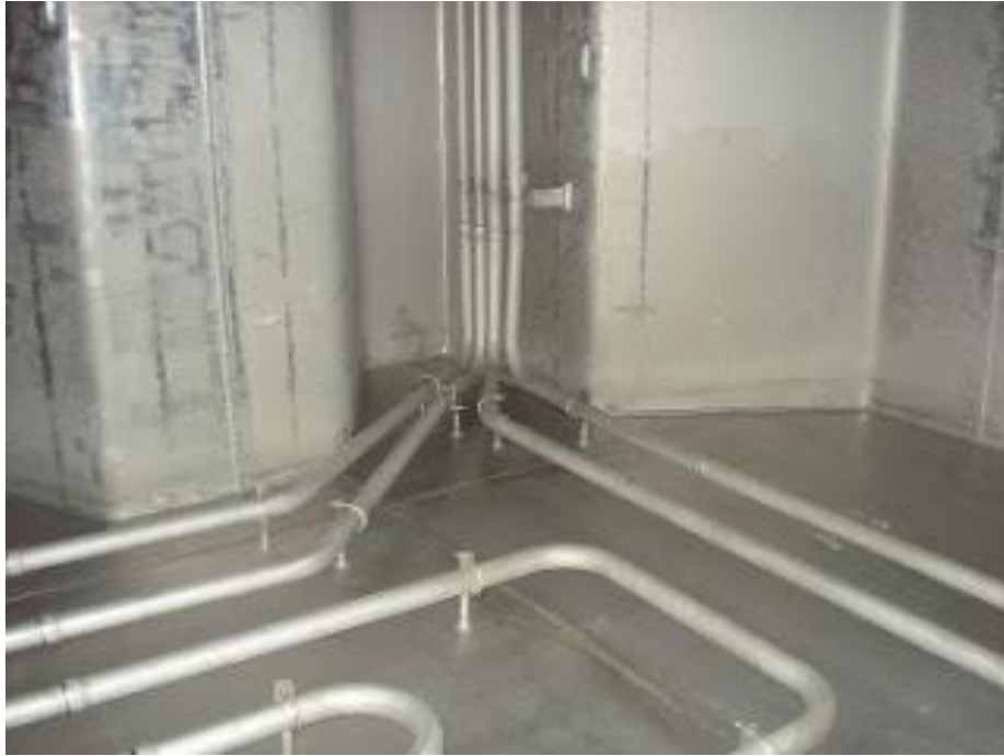
Fig. 1.5. A: Heating arrangements of a Chemical Tanker
